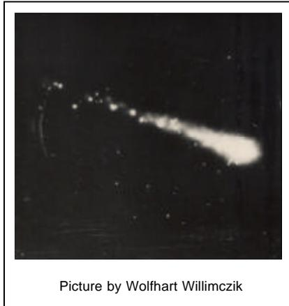
Fig. 1 shows one of the first pictures of a track of an low energetic alpha particle in my special spark chamber. The alpha particle moves from left to right.
